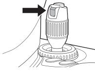
4 Adjust the observation light brightness with the observation light brightness button.
